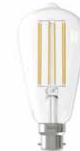
18. Clear LED Full Glass Long Filament CAL-425405, BC. (Vintage) 64 x 142mm Efficiency A+; 4W; 350 Lumens; 2300 Kelvin; Dimmable
