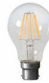
12. Clear LED Full Glass Filament GLS CAL-474501, BC. (GLS) 60 x 105mm Efficiency A++; 4W; 390 Lumens; 2700 Kelvin; Dimmable
