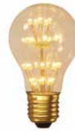
10. Pearl LED GLS CAL-474454, ES, A60 (GLS) 60 x 106mm. Efficiency A+; 1.5W; 136 Lumens; 2100 Kelvin; Dimmable
